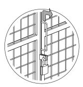
To open doors, simply lift and pull handle in one movement. (Padlock not supplied)
